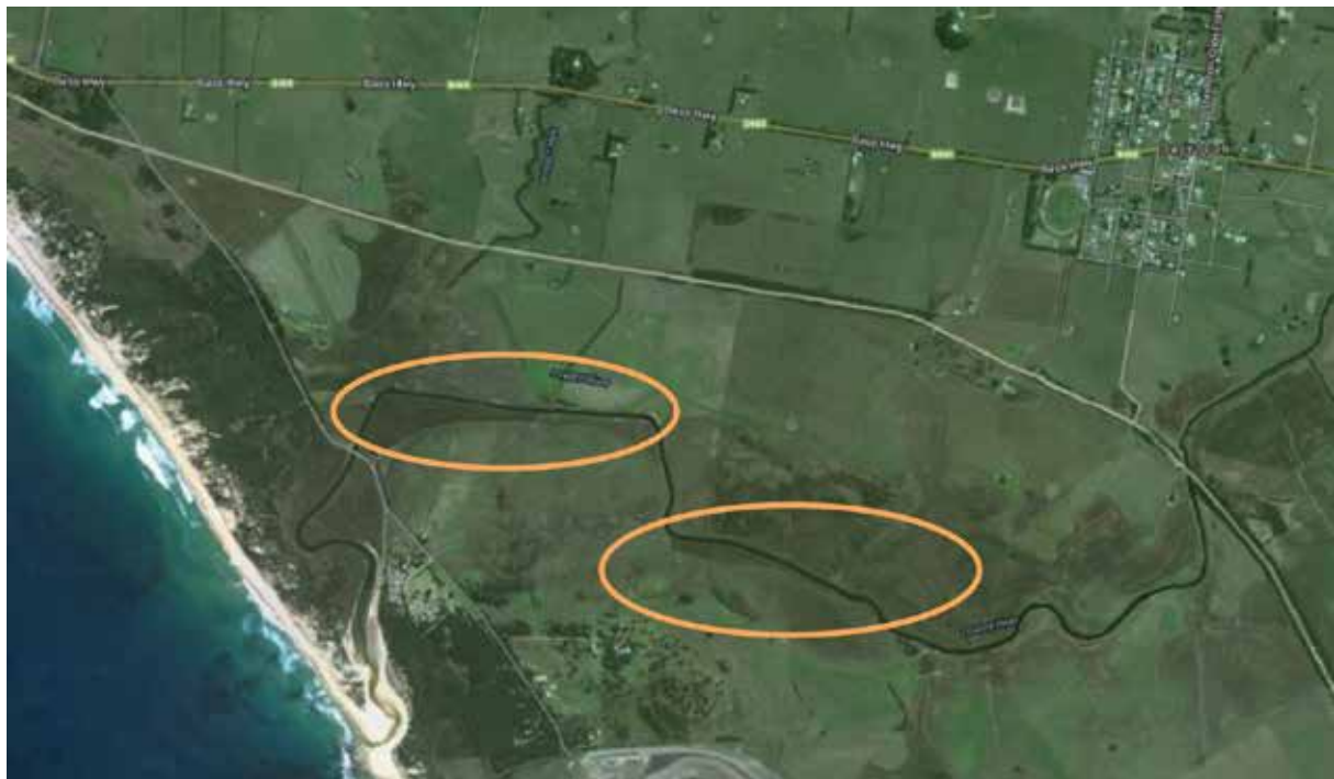
The Powlett River estuary has been straightened and channelised in several sections. Historically the estuarine wetland and swamp scrub vegetation would have spread across the floodplain, without a defined channel in many sections.
