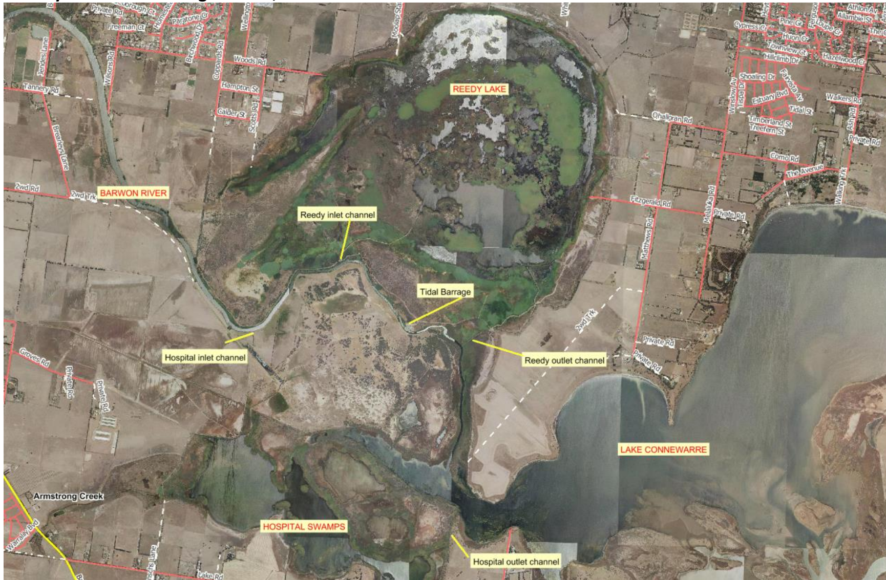
Figure 3. Lower Barwon Wetlands and watering infrastructure. The location of the watering infrastructure has guided the location of EstuaryWatch monitoring sites B7, B8 and B9.
